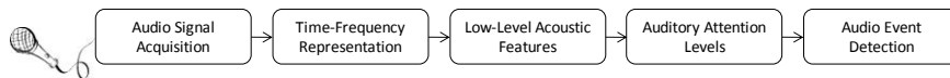
Figure 1. Block diagram of algorithm for computing normalized auditory attention levels and detecting salient and rare audio events.
