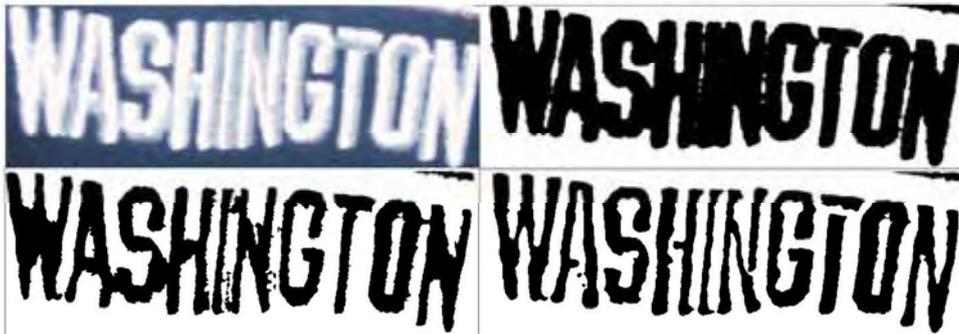
Fig. 7. Impact of varying log-Gabor bandwidth for character segmentation. Original image (top left), binary version (top right), segmentation with large bandwidth (bottom left), segmentation with narrow bandwidth (bottom right).
